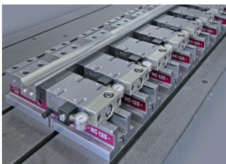
Workholding systems NC 125 with clamping force display
